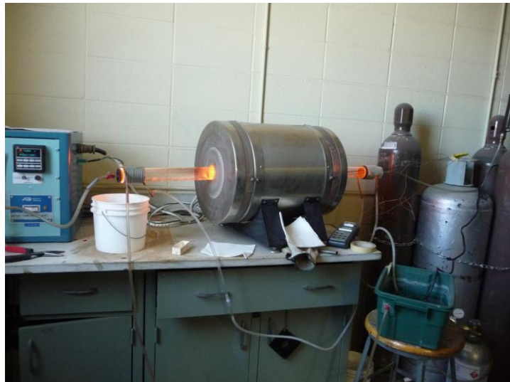
Figure 5: ATS tube furnace running at 1300°C with water cooling system.
