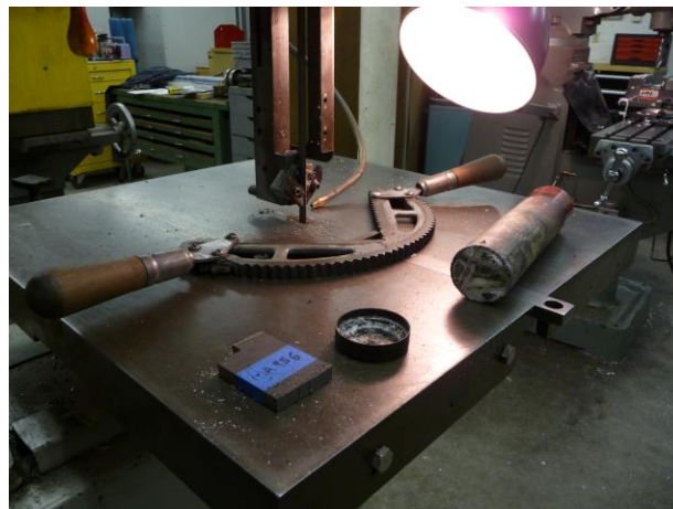
Figure 2: The DoAll band saw is pictured with the wax that lengthens the life of the band saw's blade, our MA956 parent material, and a pusher safety tool.
